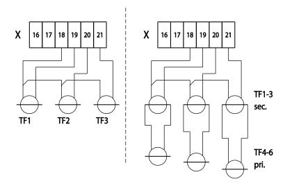
On the left side of the figure above is connection of relatively small main fuses (< 70 A), when Jäspi current transformers (TF1-3) can be used directly (depends on the size of the supply cable). On the right side of the figure is shown the connection when primary side current transformers (TF4-6) are needed and Jäspi current transformers (TF1-3) are used as secondary side current transformers.
