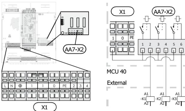
If the relays are to be used for control voltage, bridge the supply from terminal block X1:1 to X2:1, X2:3 and X2:5 on additional relay board (AA7). Connect the neutral from the external additional heat to terminal block X1:0.
