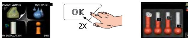
The mode for setting the indoor temperature is accessed by pressing the OK button twice, when in the start mode in the main menu.
