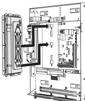
Align the two lower mountings on the reverse of the display unit with the two upper holes in the panel as illustrated.
