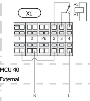
If the relay is to be used for control voltage, bridge the supply from terminal block X1:1 to X1:2 and connect neutral and control voltage from the external additional heat to X1:0 (N) and X1:4 (L).
