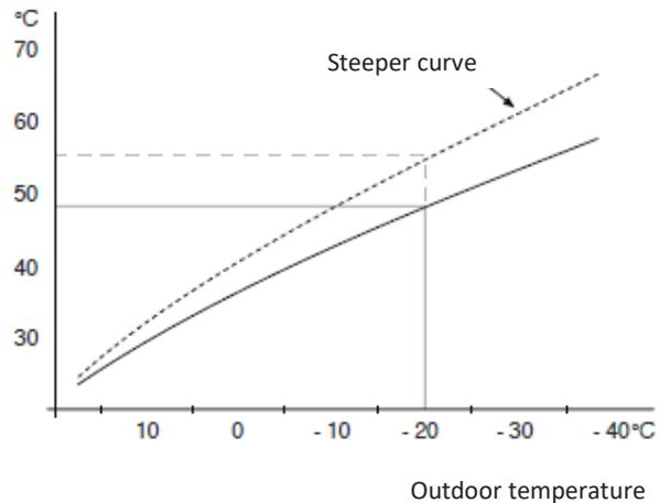
The steepness of the heat curve indicates how many degrees the flow temperature of the heating line is raised / lowered when the outdoor temperature decreases / rises. The steeper curve means a higher flow temperature at a colder outdoor temperature.
