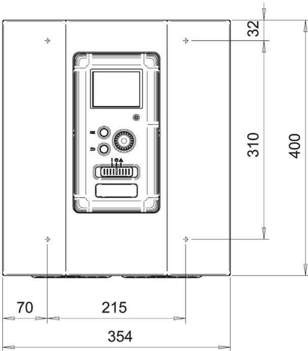
Use all mounting points and install MCU 40 upright flat against the wall without any part of the control module protruding beyond the edge of the wall.
