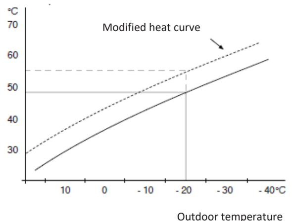
A change in the heat curve means that the flow temperature changes equally at all outdoor temperatures, for example +2 change raises the flow temperature by 5°C at all outdoor temperatures.
