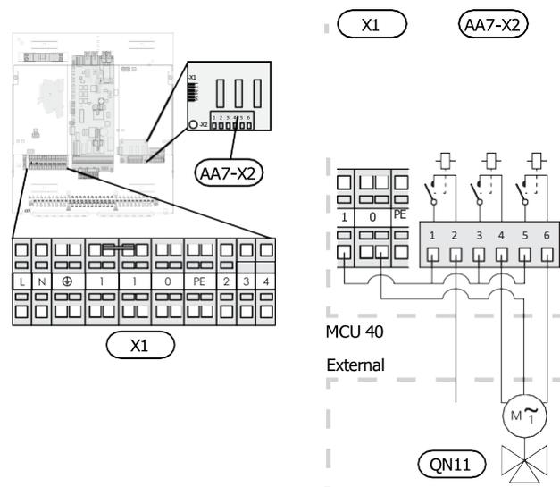
If the relays are to be used for control voltage, bridge the supply from terminal block X1:1 to X2:1, X2:3 and X2:5 on additional relay board (AA7).
