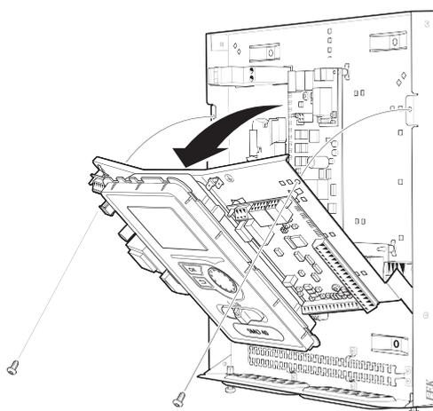
The display may need to be moved for easier access when connecting electrics. This is easily done by following these steps.
