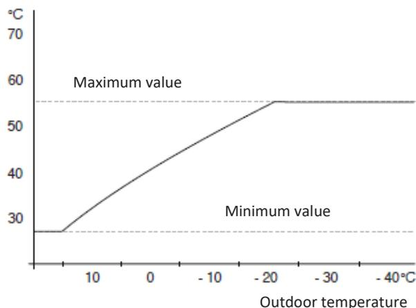
Since the flow temperature of the flow line cannot rise above the set maximum value and cannot fall below the set minimum value, the heat curve turns horizontally at these temperatures.
