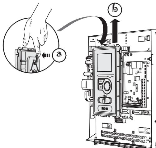
Press in the catch on the upper rear side of the display unit towards you (a) and move the display unit upwards (b) so that the mountings unhook from the panel.
