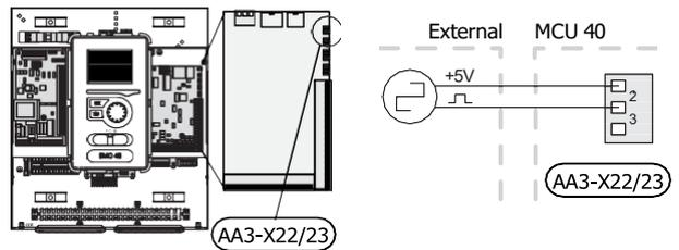
Activate the energy meter(s) in menu 5.2.4 and then set the desired value (energy per pulse) in menu 5.3.21.
