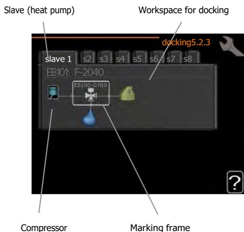
**Slave:** Here you select the heat pump for which the docking setting is to be adjusted.
