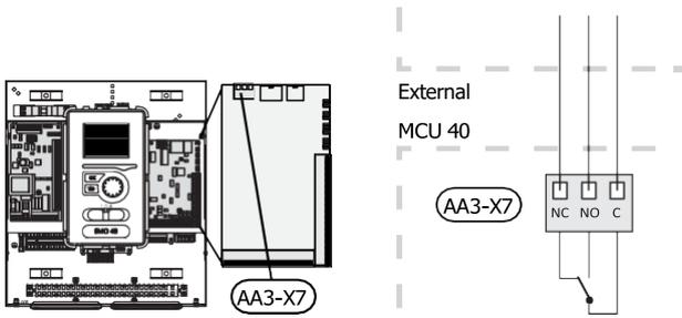
The picture shows the relay in the alarm position.
