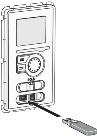
The display unit is equipped with a USB socket that can be used to update the software and save logged information in MCU 40.
