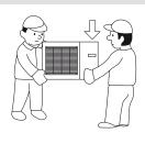
If SPLIT R6 needs to be transported across soft ground, such as a lawn, we recommend that a crane truck is used that can lift the unit to the installation location. When SPLIT R6 is lifted with a crane, the packaging must be undamaged and the load distributedwithaboom, see the illustration above.
