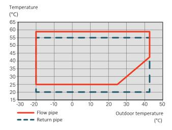
During shorter time it is allowed to have lower working temperatures on the water side, e.g. during start up.
