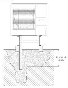
If the house has a cellar the stone caisson must be positioned so that condensation water does not affect the house. Otherwise the stone caisson can be positioned directly under the heat pump.
