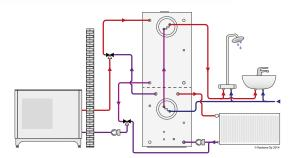
Jäspi GTV Hybrid works seamlessly with eg. a wood/oil boiler, heat pump or solar panels. The inner baffle plate ensures excellent thermal stratification.
