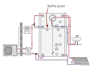
Jäspi Ovali Hybrid works seamlessly with eg. a wood boiler, heat pump or solar panels. The inner baffle plate ensures excellent thermal stratification.
