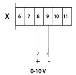
The external 0 - 10 V control property must be enabled from the software, see Menu 4.3 Input for more information. Information about voltage levels versus power steps in different modes can be found from Technical data, External control voltage (input) values and corresponding power steps in different modes.
