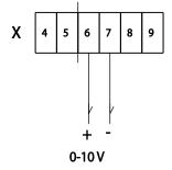
The status output 0 - 10 V property must be enabled and configured accordingly from the software, see Menu 4.4 Output for more information. Information about voltage levels versus status in different modes can be found from Technical data, Status output voltage values and corresponding status data in different modes.
