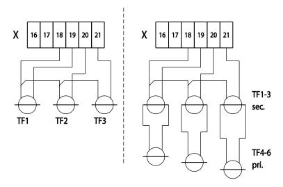
On the left side of the figure above is connection of relatively small main fuses (< 70 A), when Jäspi current transformers (TF1-3) can be used directly (depends on the size of the supply cable). On the right side of the figure is shown the connection when primary side current transformers (TF4-6) are needed and Jäspi current transformers (TF1-3) are used as secondary side current transformers.
