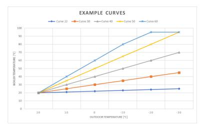
**Parallel** is parallel adjusting of the heating curve of the boiler. The value is simply added to or subtracted from the curve values. With this way, user can achieve fine adjusting for heating curve. See figure "example parallel" below.
