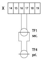
On the figure is shown the connection of primary side current transformer (TF4) and Jäspi current transformers (TF1) as secondary side current transformer.
