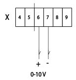
The status output 0 - 10 V property must be enabled and configured accordingly from the software, see Menu 4.4 Output for more information. Information about voltage levels versus status in different modes can be found from Technical data, Status output voltage values and corresponding status data in different modes.
