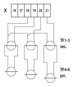
On the figure is shown the connection of primary side current transformers (TF4-6) and Jäspi current transformers (TF1-3) as secondary side current transformers.
