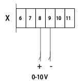
The external 0 - 10 V control property must be enabled from the software, see Menu 4.3 Input for more information. Information about voltage levels versus power steps in different modes can be found from Technical data, External control voltage (input) values and corresponding power steps in different modes.
