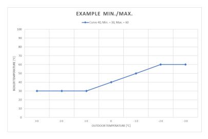
**Curve** is the heating curve of the boiler. The curve name is the value of the curve at 0 °C. The boiler temperature is adjusted against heating curve that indicates heating requirement at different outdoor temperatures. See figure "example curves" below.
